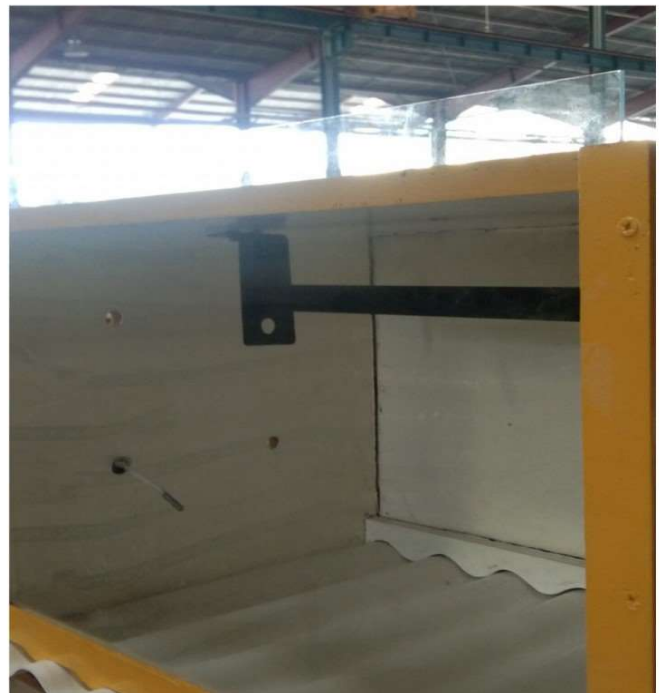
Picture A.3. Uncracked glass on PVC roof upper chamber @ time = 25 minutes
