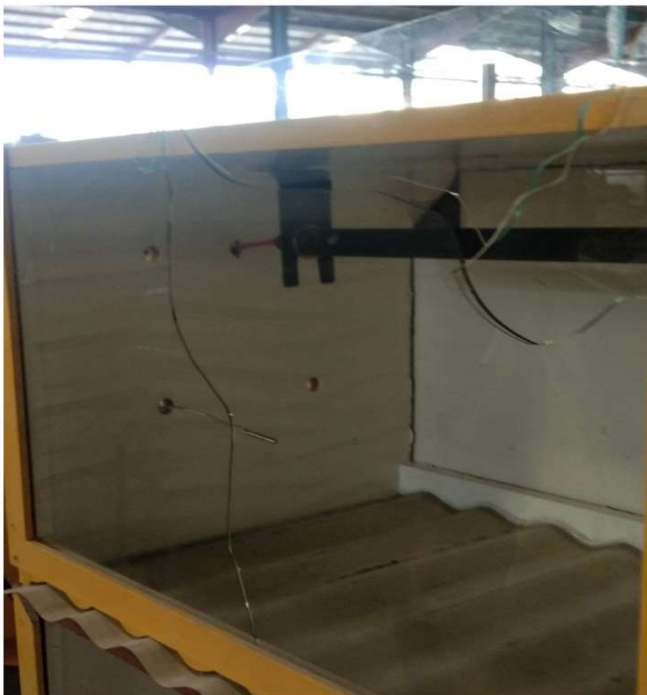
Picture A.2. Cracked glass on GI roof upper chamber @ time = 25 minutes
